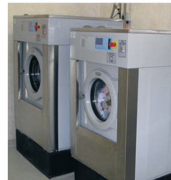
Right: Water savings are made by using Ozone washing machines in the laundry.
